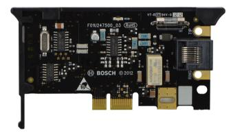
The B430 provides communication over the PSTN (Public Switched Telephone Network) by connecting the PSTN to the control panel. The module provides a single telephone jack, and easily installs into the control panel on-board plug-in module connector.
