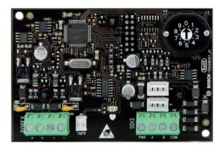
The B299 POPEX Module is an SDI2 compatible device. The module communicates to the control panel over the SDI2 bus, and provides support for up to 100 POPIT (Point Of Protection Input Transponder) devices. This occurs over a single expansion loop using two pairs of terminals.
