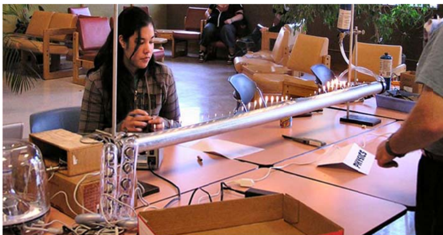
Figure 1. A "Rubens' tube" (above), designed and built by students at SCC.
