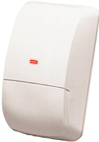
The ZX776Z PIR Intrusion Detector uses Motion Analyzer II signal processing to reduce false alarms. The detector's internally pointable mirrors and three coverage patterns provide installation flexibility. The ZX776Z includes an internal POPIT for addressable alarm and trouble signaling while communicating on the Zonex bus.
